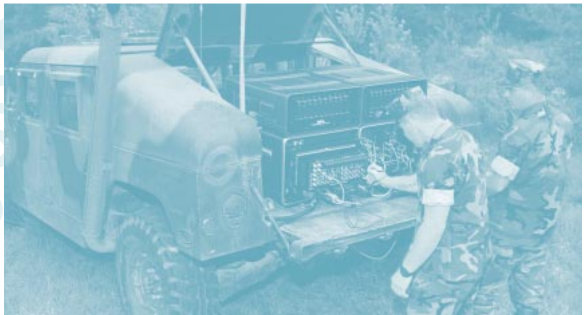
Teradyne's C-sized M910 VXI Digital Test Instrument tests electronic boards from the back of a HUMVEE.
