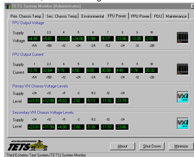
Fig. 7: Backplane voltage and current monitoring system
