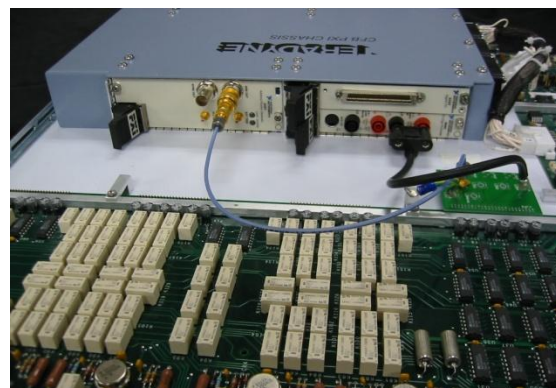
Figure 4: Connecting a PXI Instrument to the relay matrix
