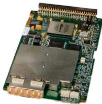
(4) front panel inputs multiplexed to the two acquisition channels. Each channel is independently capable of a 1 GHz sample rate. The 2:1 multiplexer of each channel is optimized to maintain the Ai-760 DSO's 600MHz input bandwidth for all inputs. As a result integrators can wire each of the two acquisition channels to their ICA and still have a second probe input signal for each channel.
