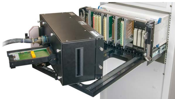
Figure 4: Example of a Test Fixture That Also Uses External connections.
