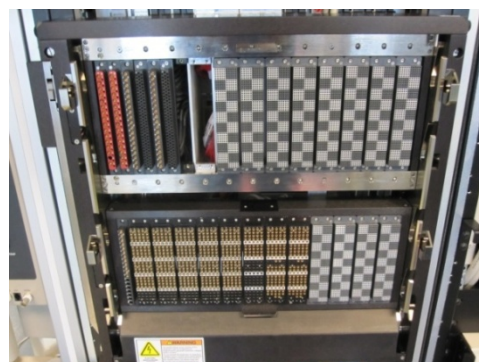
Figure 2: One-Tier VPC 90 Interface Expanded to Incorporate a Second Tier of Pins.
