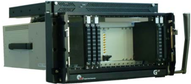
Figure 17: 1U PC Controller Positioned above the PXI Chassis.
