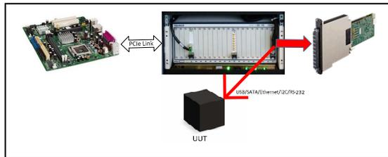
Fig. 2. Example peripheral instrument test setup
